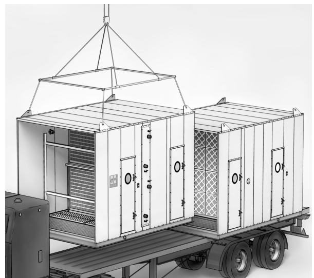
Figure 6: Lifting of a unit with roof mounted lifting brackets. Image is misleading. Most likely, the unit shown weighs more than 2000 lbs., which is the capacity for 4 lifting brackets.
