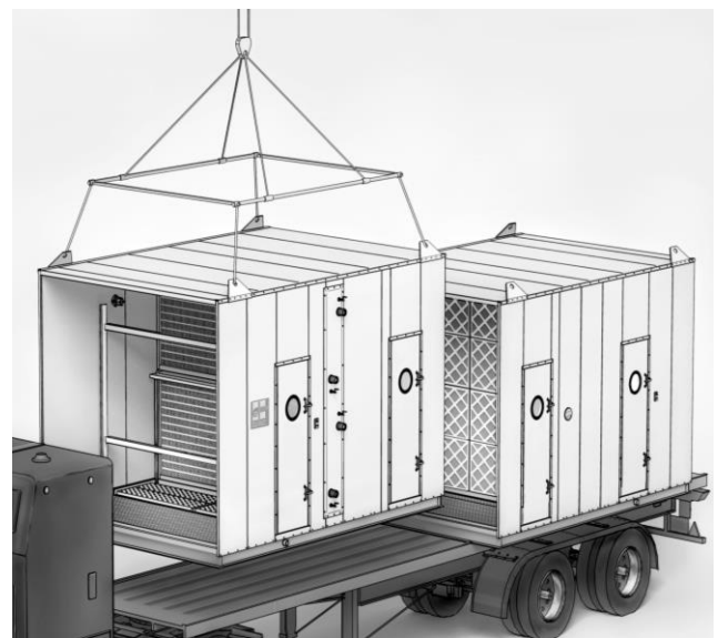
Figure 4: Lifting of a unit with roof mounted lifting brackets.
